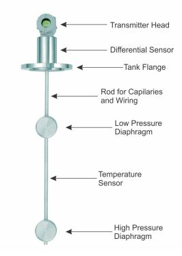
The distance between the diaphragms and the variation of the filling fluid in the capillaries that transmit the pressure from the diaphragms to the capacitive sensor must be considered.
